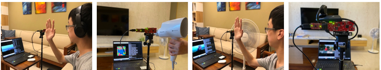
Figure 16: Four types environmental interference scenarios. From left to right are Bluetooth (headset), electromagnetic waves (hair dryer), fan swiping and millimeter-wave radar.
