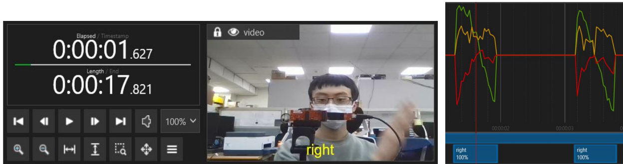
Figure 10: Data labeling, the left is the video track and the right is the waveform track. Labels are annotated by human inspection with the aid of video to avoid mislabeling.
