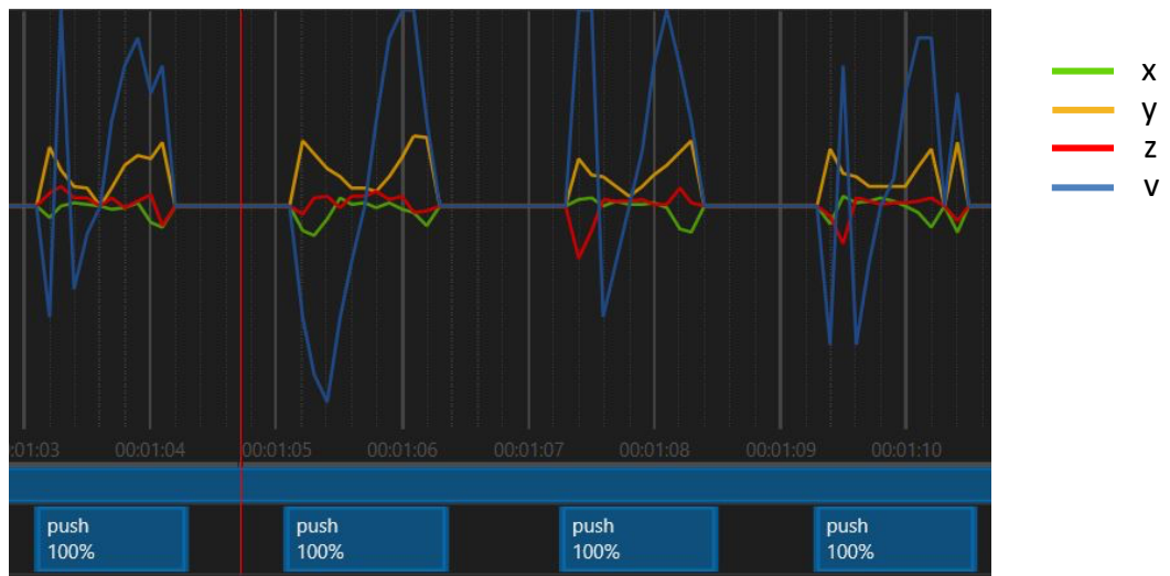
Figure 6: Cartesian coordinate and velocity (blue line) waveform of push gesture at different speeds. Velocity waveform is not a key feature.
