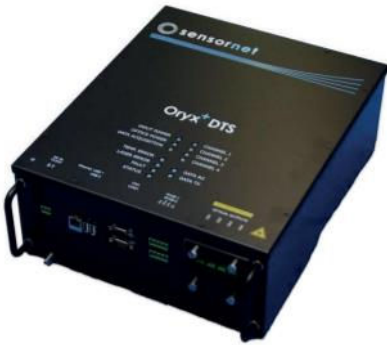
Fig.13: Photograph of the DTS sentry used (Sensornet, DataSheet v.2, 2020).
