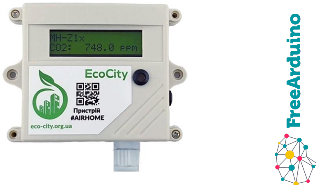
Figure 2.1. Air quality monitoring sensor, that has been developed by Ukrainian company.
