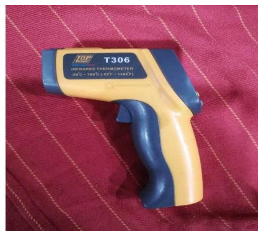
Figure 4: An Infrared thermometer was used to measure temperature.
