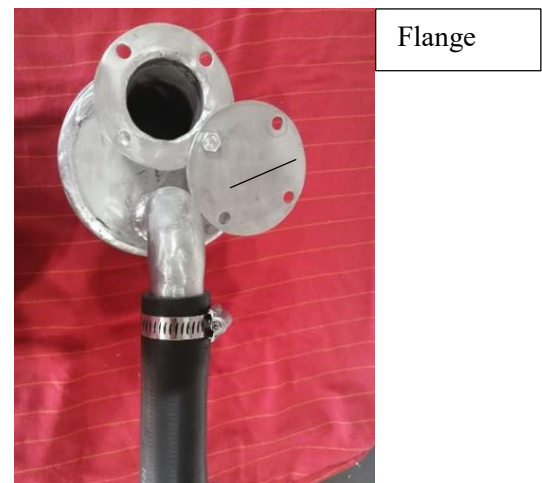
Figure 21: There is a blank flange that can be screwed and unscrewed to inject plastic.
