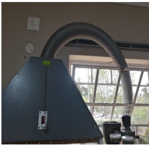
Figure 33: The fume cupboard allows the gas to escape the room.
