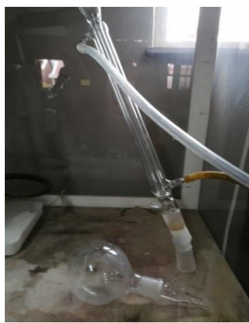
Figure 35: The condenser has a tube where water passes over the inner tube.
