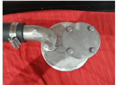
Figure 19: The tube that the gas will flow through has a hose clamp attached to it.
