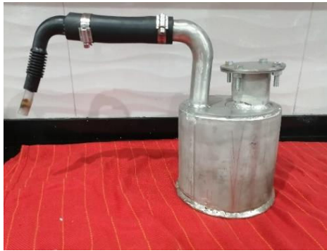
Figure 18: The vessel was built with two orifices.
