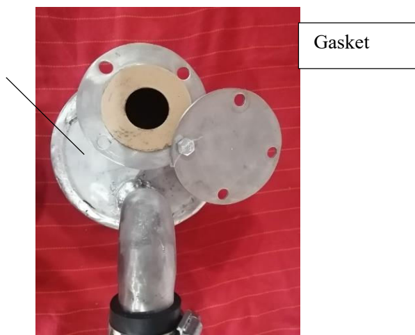
Figure 20: The gasket is used to stop the gas from escaping.
