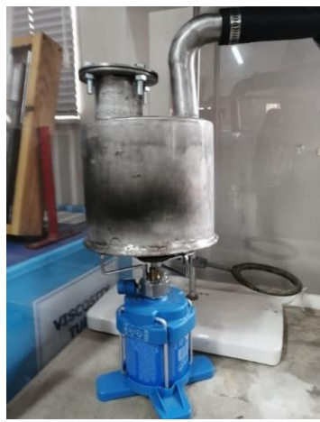
Figure 34: The vessel was placed onto a gas stove, and the process was repeated for plastic fuel and coal.
