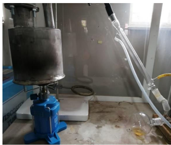
Figure 36: Two pipes are placed onto the outer tube of the condenser to allow water through.
