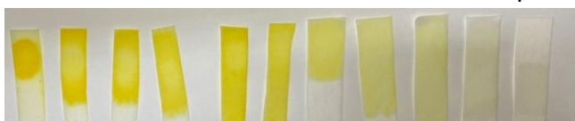
Figure 8 Our handmade fast test paper (prepared by absorbing the buffer-contained colorimetric reagent), which was useful to detect the hydrogen peroxide
