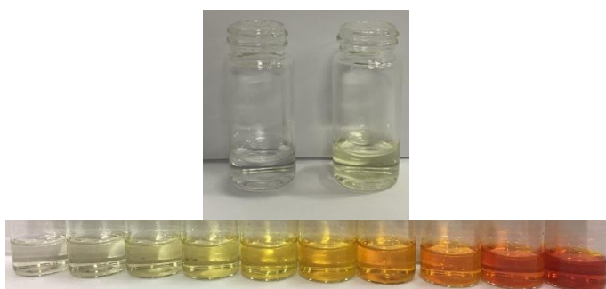
Figure 1 Yellow or orange color refers to a positive response if titanium (IV)-contained colorimetric reagent reacted to hydrogen peroxide
