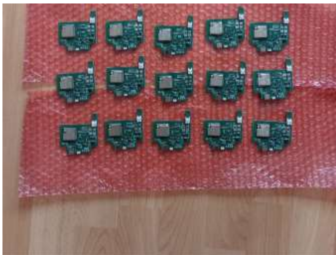
Figure 14: The ordered circuits assembled with small components
