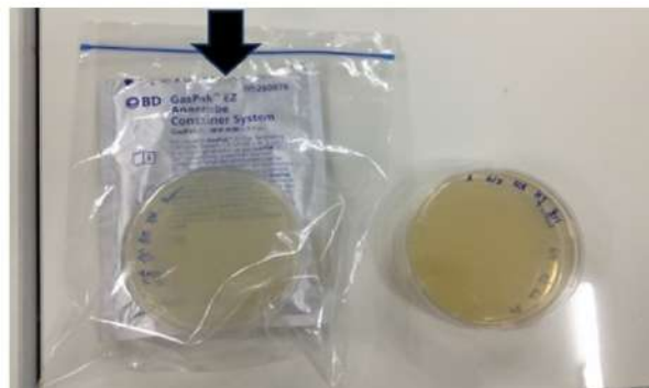
[Fig.4] Oxygen-Absorbing Carbon Dioxide-Releasing Patch Placed in a Sealed Zipper Bag with the Culture Medium
