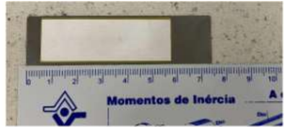
Figure 6 – Piezoelectric device used in the experiment.
