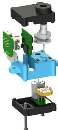
Fig. 2 MG-90I servomotor exploded view
