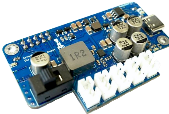
Fig. 8 PCB for Power Management
