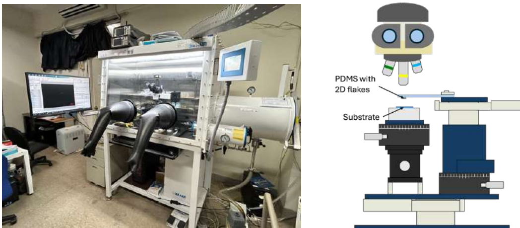
Figure (12) | Glove box for 2D transfer system (left), and a schematic structure of the system.
