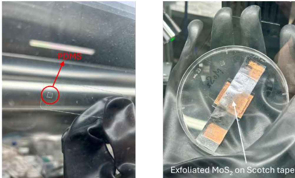
Figure (11) | Thin film of PDMS on a glass slide (left), and the exfoliated MoS 2 on a strip of Scotch tape (right).
