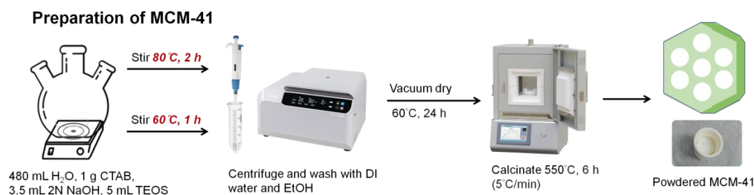
Figure 2. Schematic illustration showing the preparation of MCM-41
