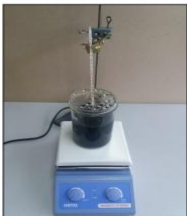
Figure 11. Mixing of Corn Cob Ash with NaOH Solution
