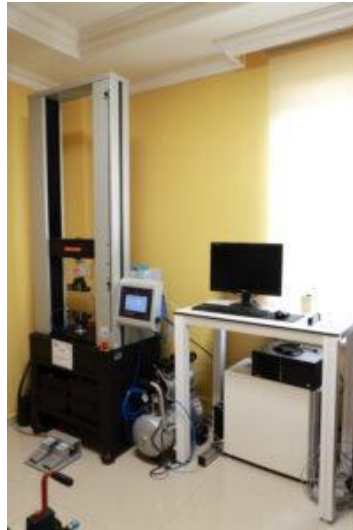
Figure 10 - Devotrans CKS-III Tensile, Compression, and Bending Test Machine
