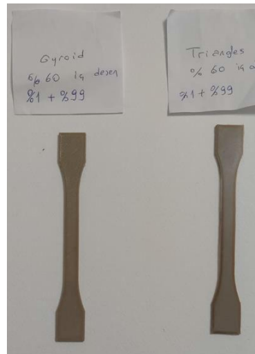
Figure 17 - ISO 527-4 Tensile Test Specimen
