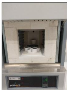
Figure 10. Burning of Corn Cobs in the Furnace
