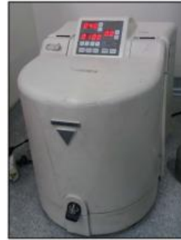
Figure 16. Mill Used for Grinding and Mixing Processes
