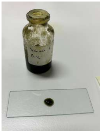
Figure 19 : Spreading Ability Test Results of Variant 1
