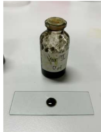
Figure 20 : Spreading Ability Test Results of Variant 2
