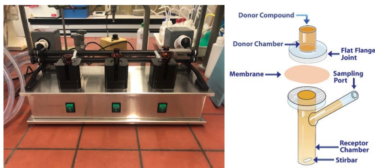
Figure 4. Franz diffusion apparatus with 3 cells (left), breakdown of a single cell (right) [xxiv].
