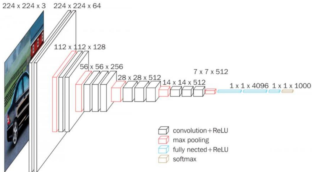
**Pic13. Model structure of VGG16**
