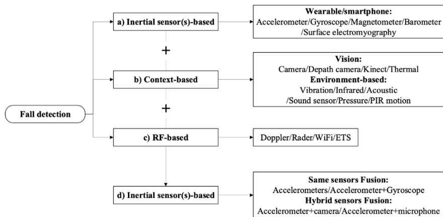
*Pic7. Current solution for fall detection*
