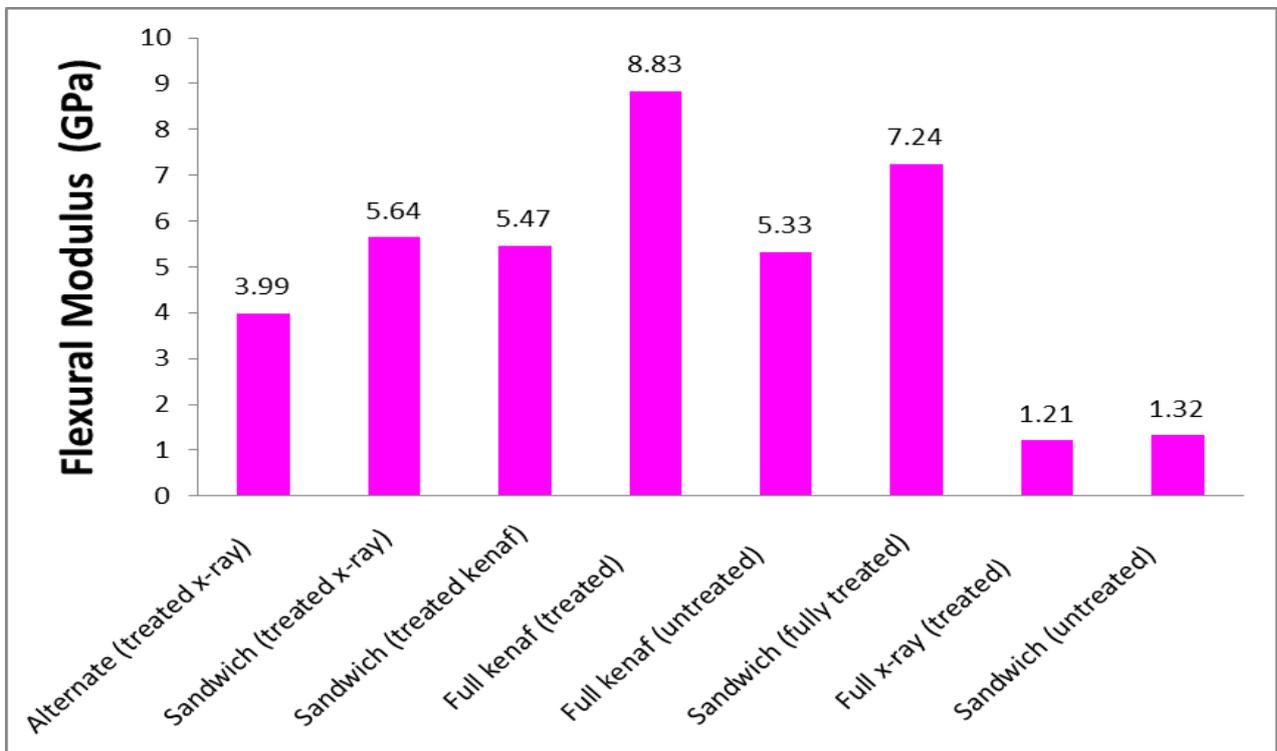
Graph 4 : Flexural modulus of composite kenaf and x-ray film waste
