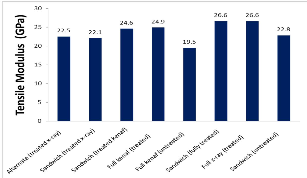
Graph 2 : Tensile modulus of composite kenaf and x-ray film waste
