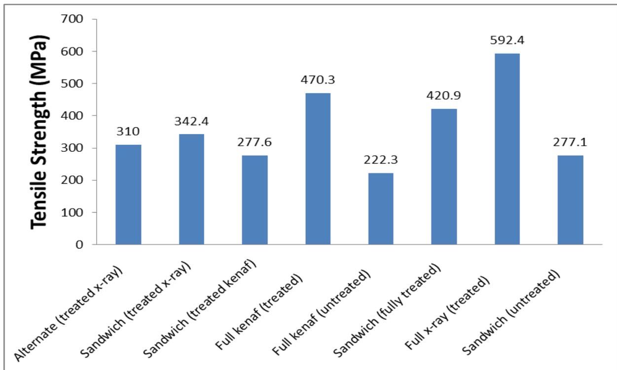
Graph 1 : Tensile strength of composite kenaf and x-ray film waste
