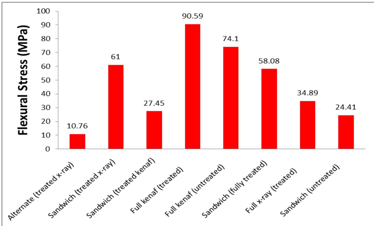
Graph 3 : Flexural stress of composite kenaf and x-ray film waste
