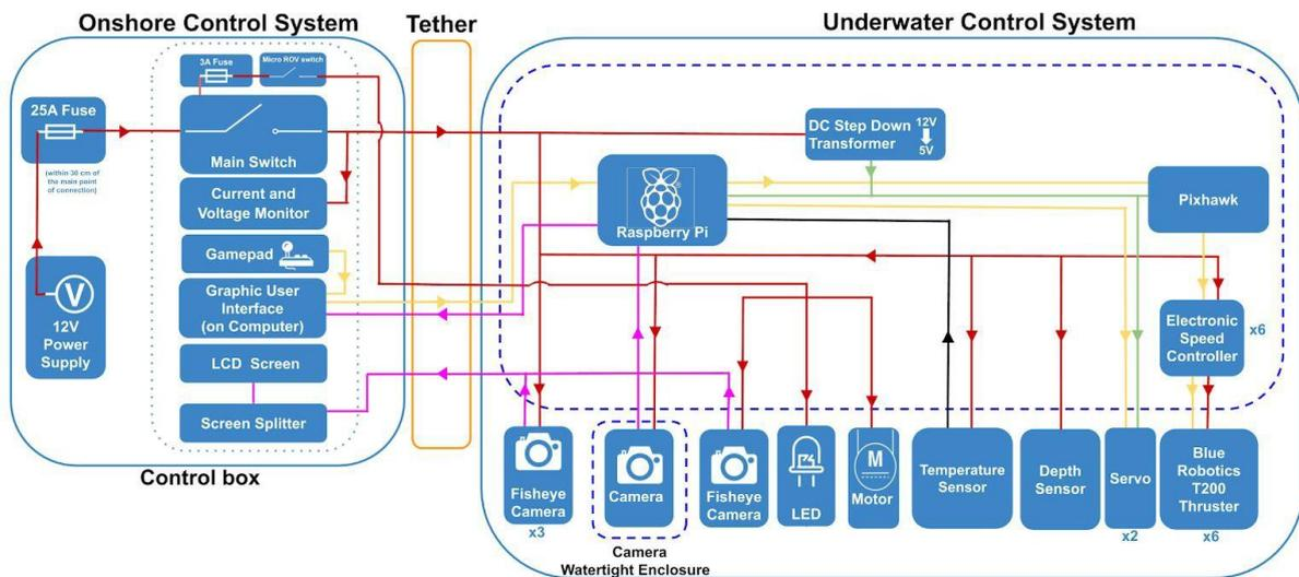
fig.6 Planned System Integration Diagram (SID)
