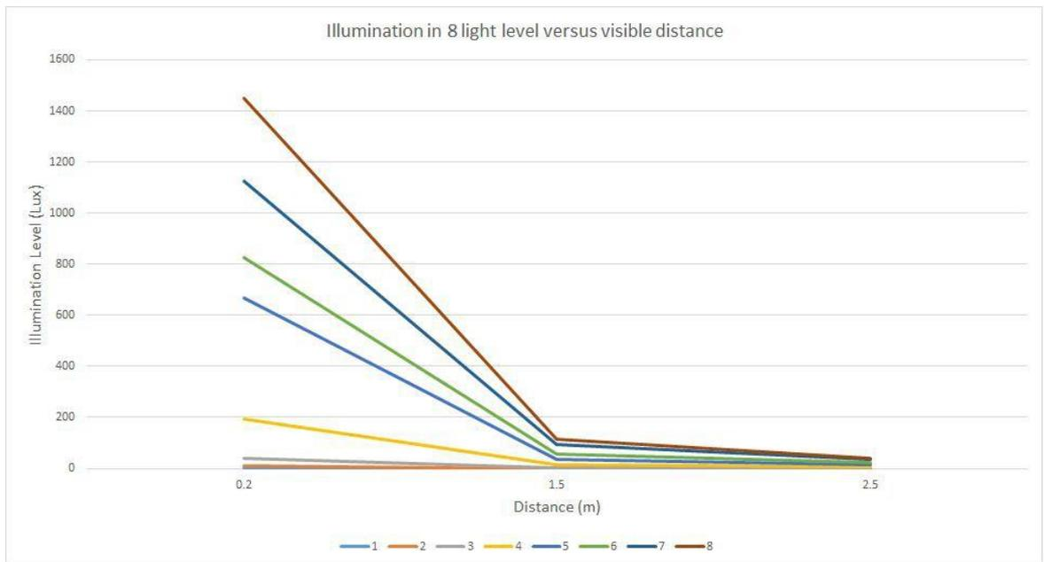
fig.14 The visibility performance through the camera with 8 adjustment of the luminosity of the LED lights
