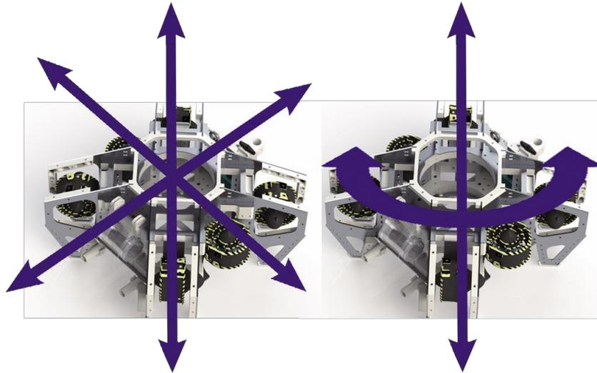
fig.11 Multi-directional movement of the vehicle
