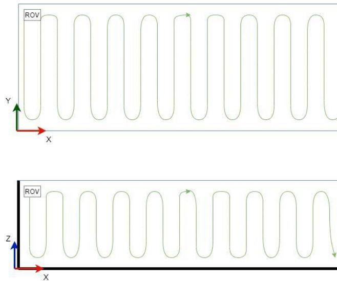
fig.4 above diagram: Aerial view of the autonomous searching route
