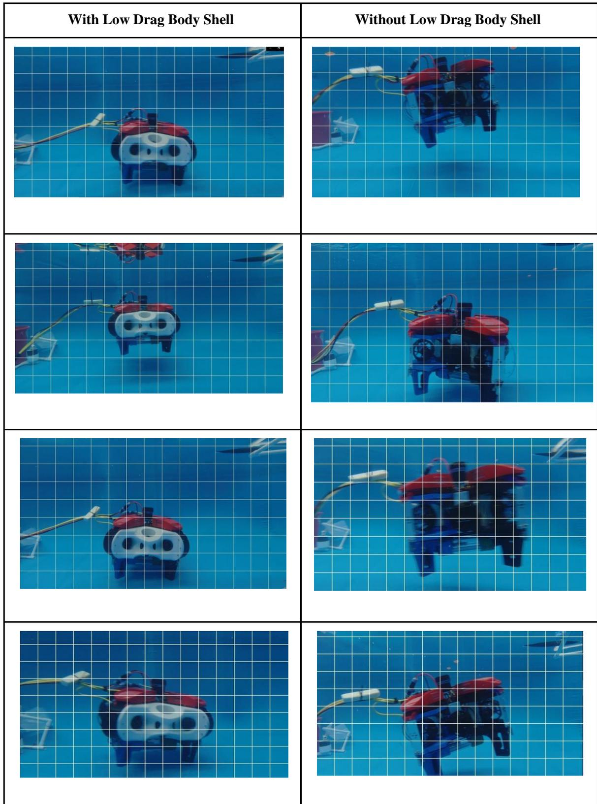
fig.18 Movement stability comparison
