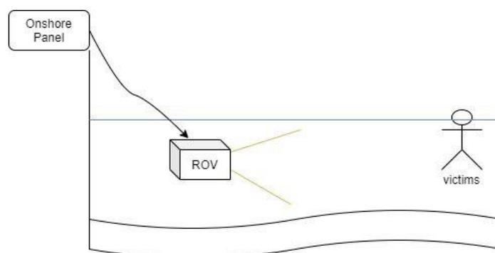
fig.3 Tethered ROV searching for victims in the flooding condition with LED lights deployed
