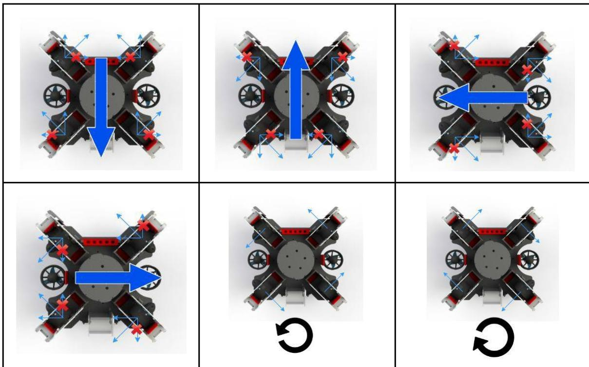
fig.13 The arrangement of thrusters leading to the multi-directional movement of the ROV
