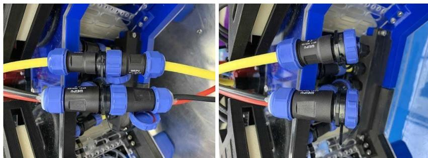
fig.7 Waterproofed quick-release plug
