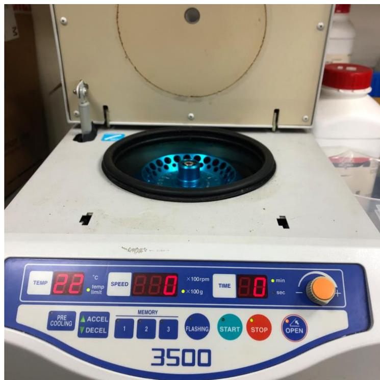
**Figure 8. Centrifuge.** The centrifuge was used for the removal of excess supernatants after the conjugation of anti-Dengue rabbit antibody on FNDs.
