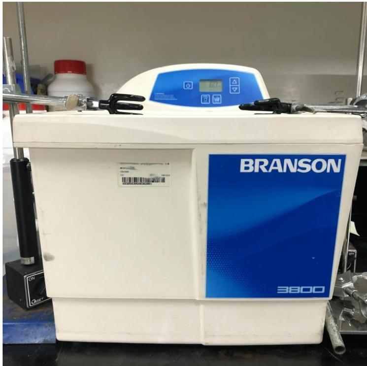
**Figure 7. Ultrasonic Bath.** The ultrasonic bath was used for the agitation of FNDs and the mixing of FNDs with anti-Dengue rabbit antibody.
