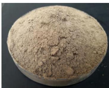
Diagram 6 : Fly ash collected from Manjung coal fired power plant
