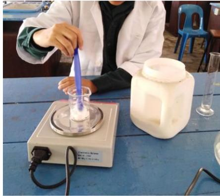
Diagram 9 : Weight a substance based on mixture proportions.
