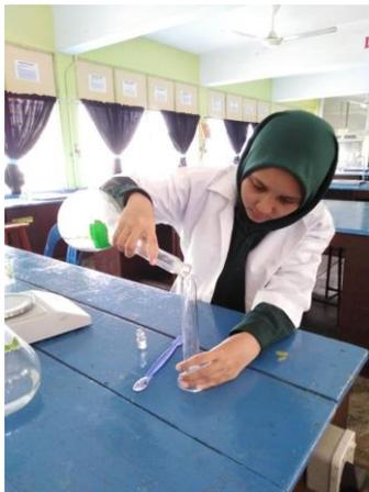
Diagram 8 : Measure the volume of HCl used form treatment
