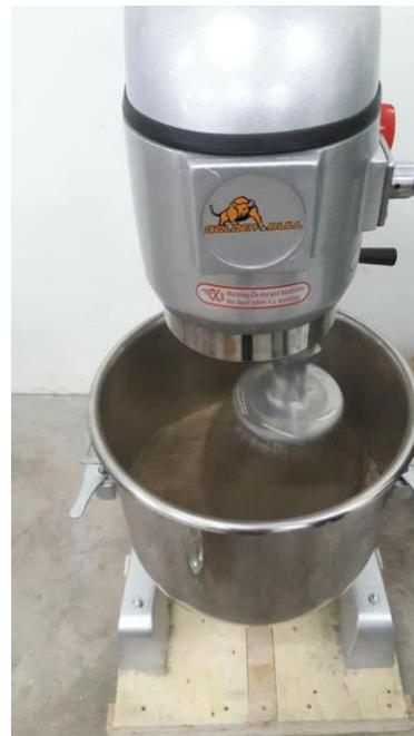
Diagram 10 : Fly ash, fine aggregate and paper mill sludge ash (if any) were mixed in a bowl mixer for mixing process .
