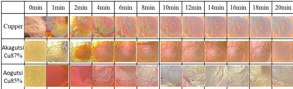
**Fig. 4** Color change of brass foil and copper foil on the hot plate
