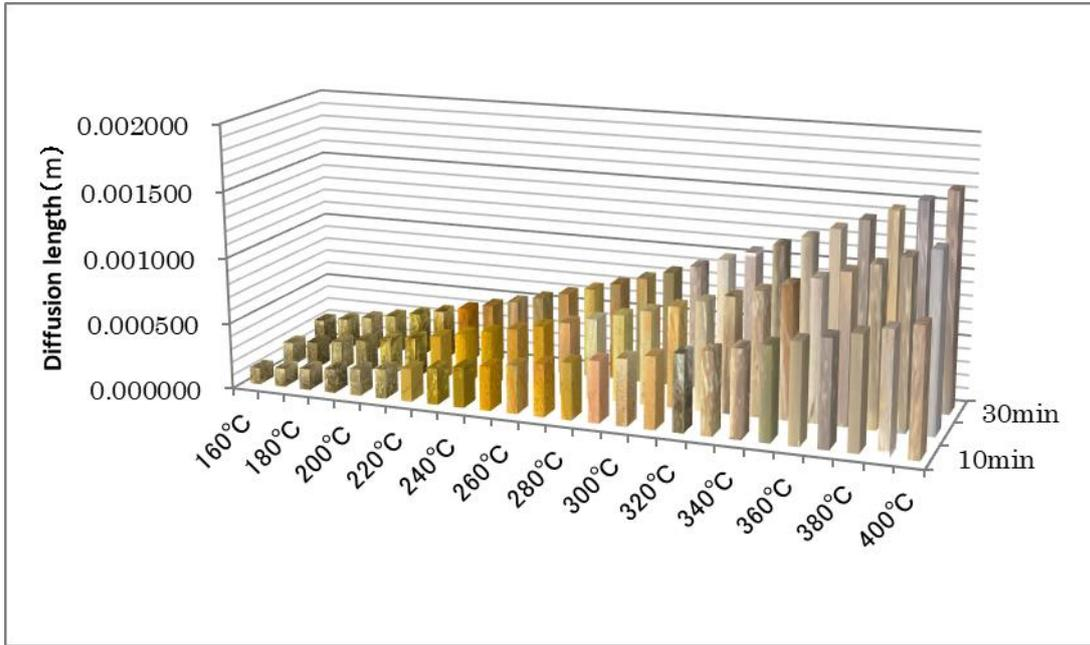
**Fig. 11** Relationship among heating time, temperature, diffusion length of oxygen atoms, and color change in Akaguchi.
