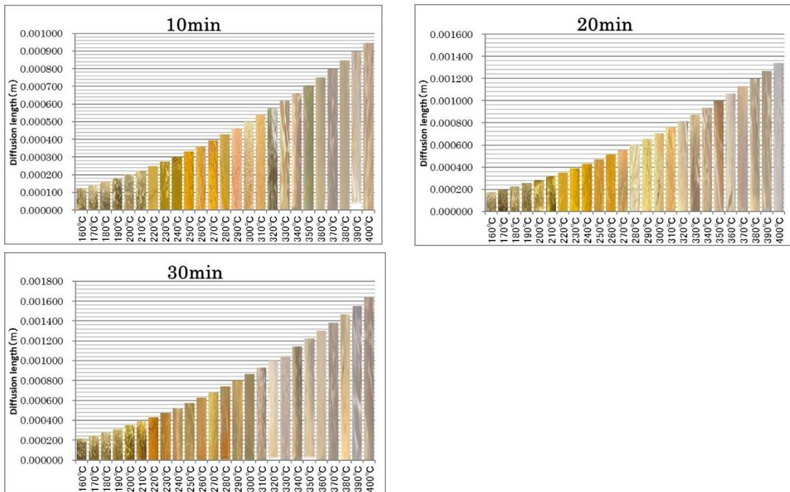
**Fig. 12** Relationship between temperature and diffusion length in Akaguchi when time is kept constant
