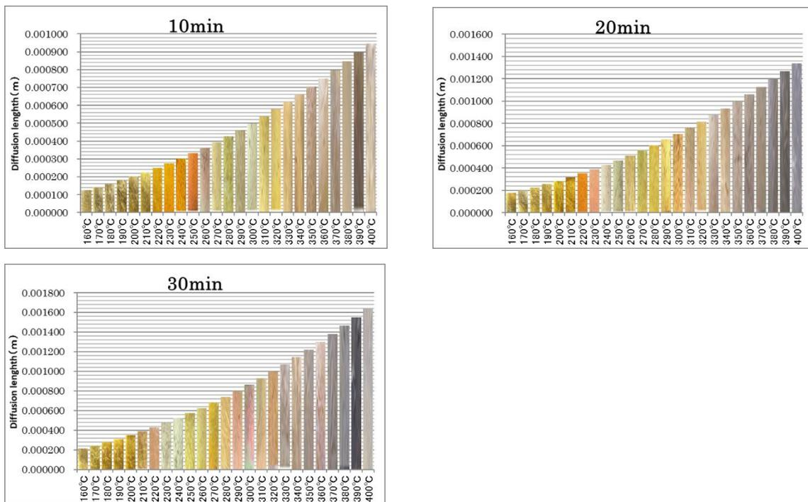
**Fig. 8** The relationship between the temperature and diffusion length in Aoguchi
