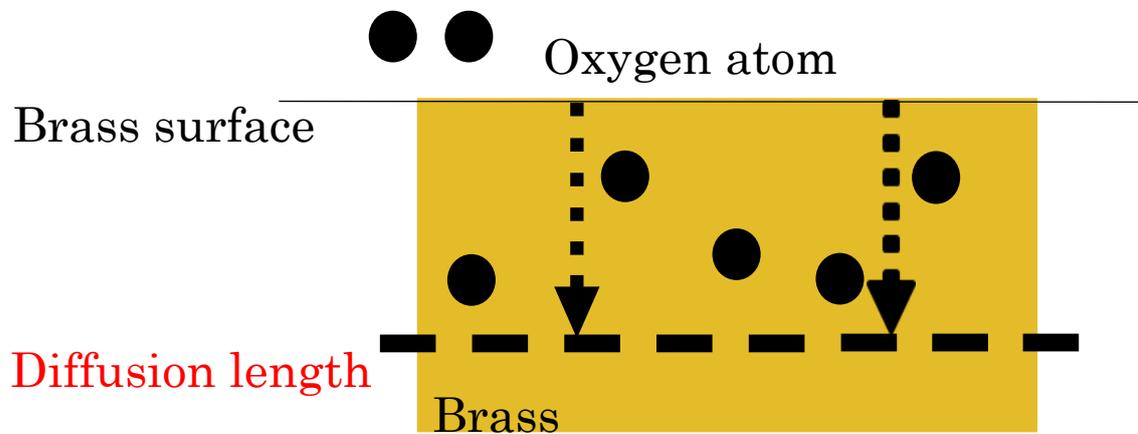
**Fig. 6** Penetration and diffusion length of oxygen atoms on brass surface
