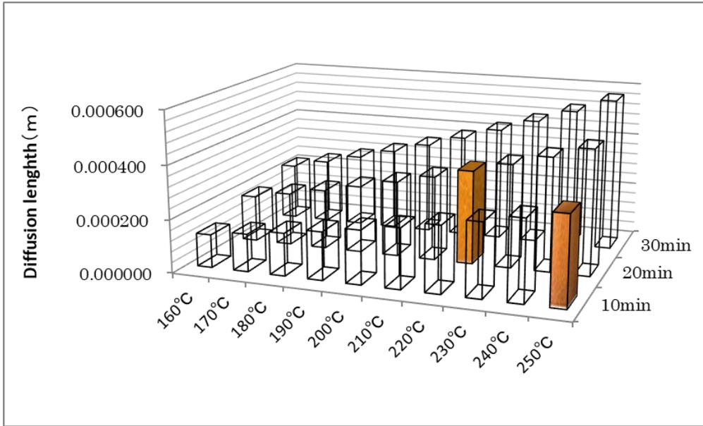
**Fig. 9** Diffusion length of oxygen atoms around the heating temperature and heating time.
