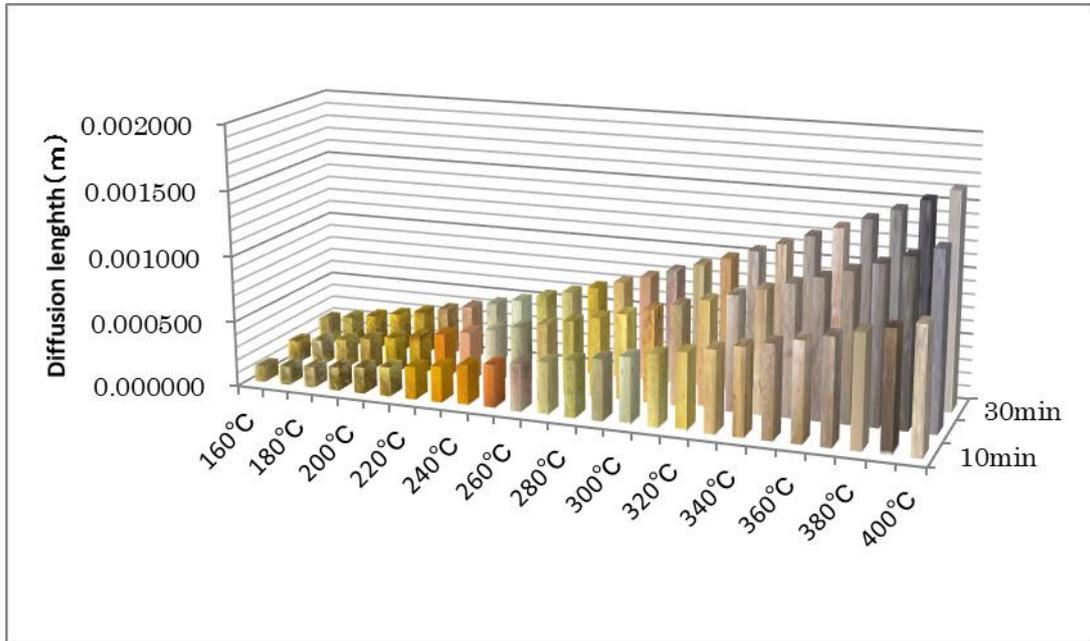
**Fig. 7** Relationship among heating time, temperature, diffusion length of oxygen atoms, and color change in Aoguchi
