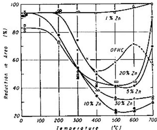
**Fig. 5** Cross-sectional shrinkage vs. temperature curve of brass at low temperature test
