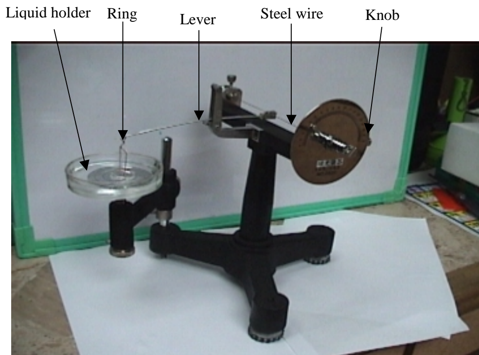
Photo 1. Setup of Du Noüy surface tensiometer
