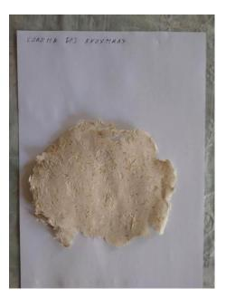
*Picture 3.3*\* Paper which was made with the addition of pumkin seed shells without starch
