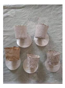
*Picture 3.10*\* The ready pots. View from the side. The top line of pots were made without using cheesecloth, the bottom line of pots were made with using bandage
