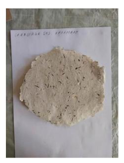
*Picture 3.5*\* Paper which was made with the addition of sunflower seed shells without starch
