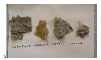
*Picture 3.8*\* Samples of paper after 20 minuts spent in water
