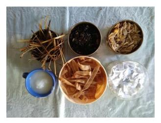
*Picture 3.1*\* Samples of raw materials for research – agricaltureal waste (straw, bean husks, sunflower and pumpkin seed shells), waste paper and starch
