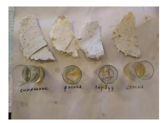
*Picture 3.7\** Samples of paper were placed in water at temperature approximately equal to  $20^{\circ}$  C
