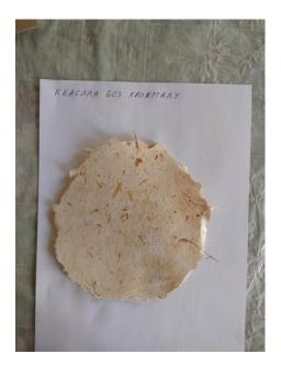
*Picture 3.4*\* Paper which was made with the addition of bean husks without starch
