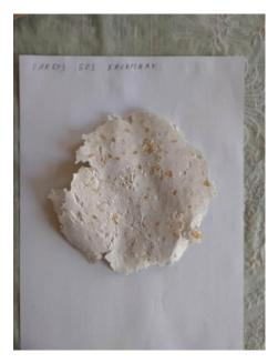
*Picture 3.6*\* Paper which was made with the addition of pumkin seed shells without starch
