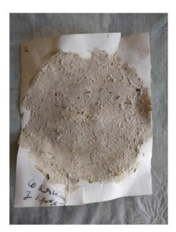
*Picture 3.2*\* Paper which was made with the addition of sunflower seed shells and starch
