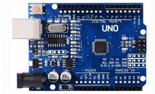
Fig. 2.3 Arduino Uno board Fig. 2.4 MQ-135 gas sensor (NO 2 , CO 2 , CO, CH 2 O)
