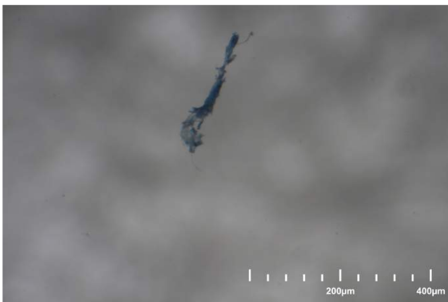
Figure 24 Frayed fiber fragment (blue) of an unworn surgical mask on cellulose filter (gray-white).
