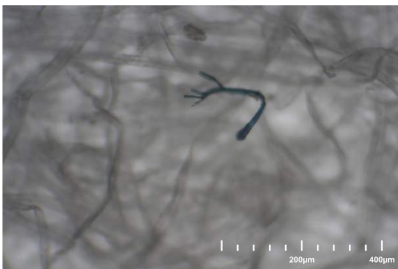
Figure 20 Fiber fragment (blue) with split and branched end (surgical mask 8.5h school) on the cellulose filter (gray-white)
