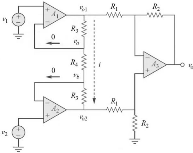
As An instrumentation amplifier (IA) is used to provide a large amount of gain for very low-level signals, often in the presence of high noise levels. The major properties of IAs are high gain, large common-mode rejection ratio (CMRR), and very high input impedance
