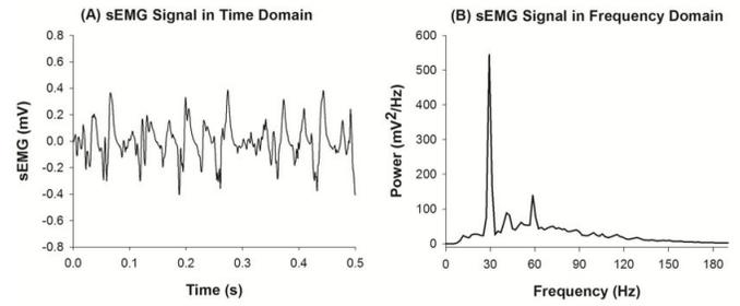
Fig. 9. Surface electromyography (sEMG) signal of the Vastus Lateralis during wholebody vibration at 30 Hz illustrated in (A) the time domain and (B) the frequency  $f_0$  domain. In the frequency domain, excessive spikes are visible at the vibration frequency and its multiple harmonics.
