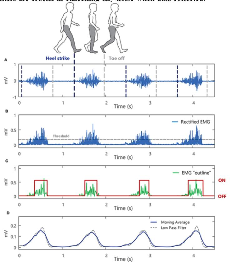
Fig. 13. Mechanism of electrical pulses From sEMG to captured it
