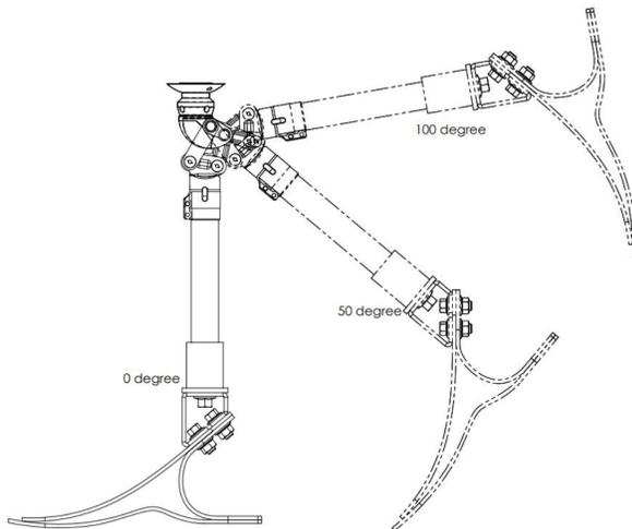
Real-life motion modeling for the prosthetic leg with 100 angel of movement as shown in (fig 5).
