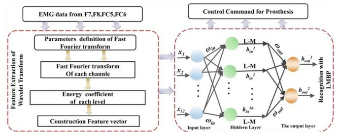
As shown in (fig 1) The fast Fourier transform (FFT) steadily transforms a time-domain signal into different frequency scales. Hence, the FFT was selected to extract EMG features in this study. The statistical parameter of FFT energy coefficients can be obtained using the following equation:
