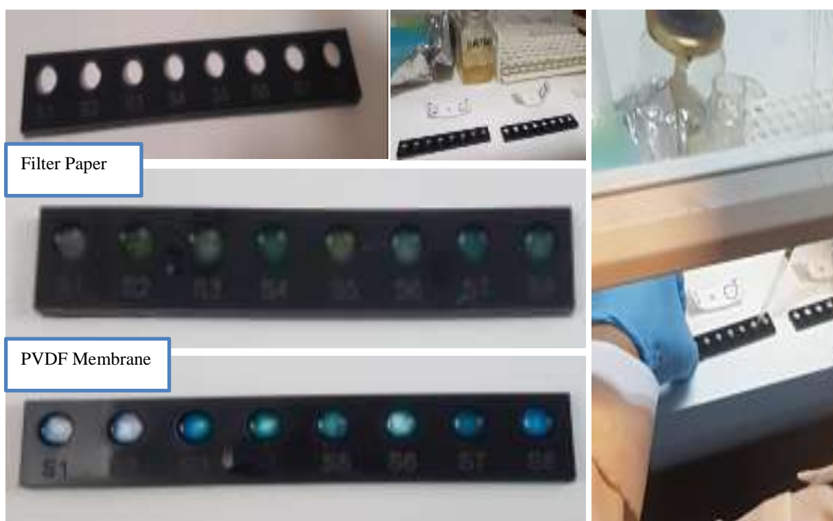
Figure 16. Determination of bacteria at different concentrations with the microchip biosensor platform
