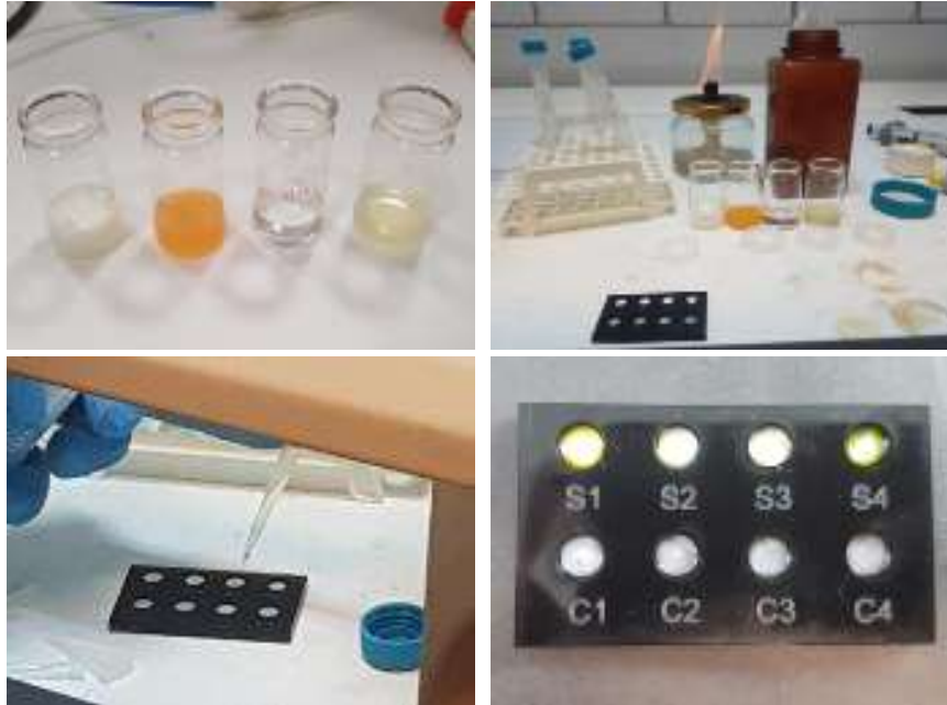
Figure 13. Detection of bacteria in various beverages with the microchip biosensor platform
