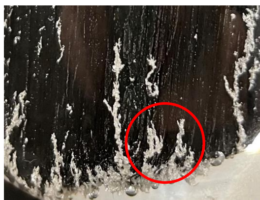
Fig. 7 Silver (dendritic crystals) deposited from bincho charcoal
