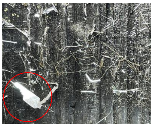
Fig. 6 Silver (planar crystals) deposited from cedar charcoal
