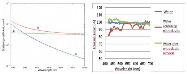
**Figure.4.8** A)Rayleigh scattering (1),Mie scattering (2),Combination of Mie and Rayleigh scattering equations (3) (Petrov,2012). B) Transmission display chart where before and after plastics were removed from water.
