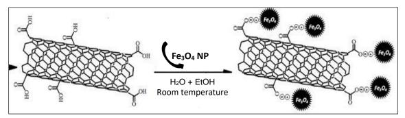
Figure.3.2 m-CNT 's synthesis reaction (Sadegh vd., 2014; Sadegh vd., 2018).
