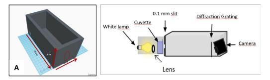
**Figure.3.1** a) The 3D design of the spectrometer that has been made with TinkerCad, b) Schematic representation of the spectrometer(Original).
