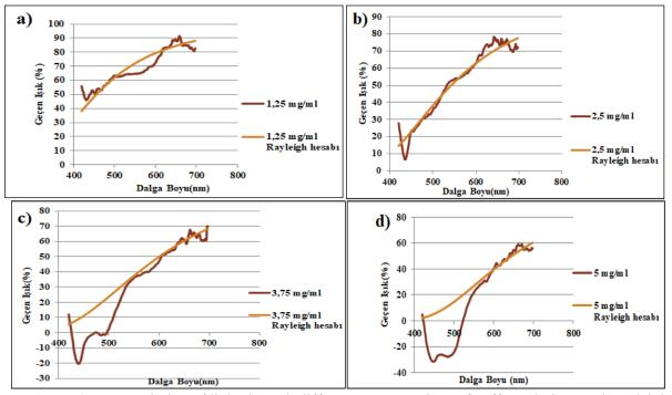
Figure.4.5 Transmission of light through different concantrations of coffee solutions and Rayleigh scattering calculations. a) 1,25 mg/mL b) 2,5 mg/mL c) 3,75 mg/mL d) 5 mg/mL
