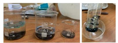
**Figure.4.6** A)Steps of Magnetic Separation. B) The picture of accumulated microplastics on the magnet after the magnetic separation from the water.
