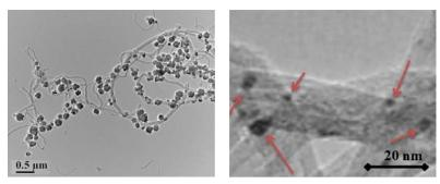
Figure 2.10. Image of synthesized material of CNT and  $Fe_3O_4$  NP's at electron microscope (TEM) (Saber-Samandari vd., 2016; Sadegh vd., 2018).
