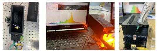
**Figure 4.1** Constructing and connecting the spectrometer with the Theremino software (orijinal). And Theremino software was established and measurements were initiated (Figure 4.1). As seen in Figure 4.2.A, the peak points in the measurement of the spectrometer taken with the sodium lamp are at wavelengths of 589.0-589.6 nm. Thus, the theoretically expected value was obtained and our spectrometer was calibrated.
