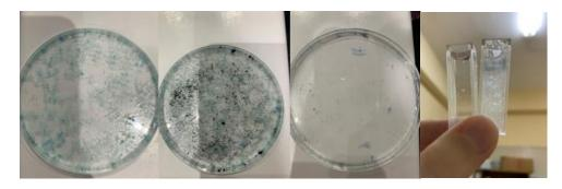
**Figure.4.7** A) The sample containing HDPE microplastics B) Suspension where m-CNT is added. C) Sample after the microplastics are removed D) Cuvettes with samples before and after the microplastic removal.
