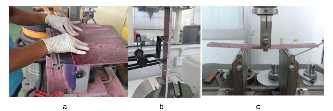
Fig. 1. Testing process: a) specimen cutting; b) tensile test setup; c) 3-point bending setup
