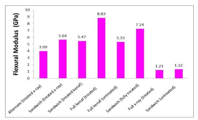
Graph 4 : Flexural modulus of composite kenaf and x-ray film waste
