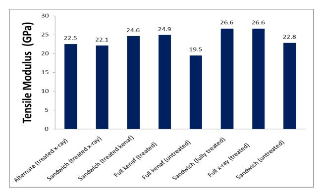
Graph 2 : Tensile modulus of composite kenaf and x-ray film waste
