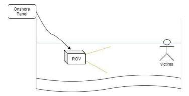
fig.3 Tethered ROV searching for victims in the flooding condition with LED lights deployed
