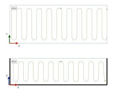
fig.4 above diagram: Aerial view of the autonomous searching route below diagram: Dive in and float up of the autonomous searching route
