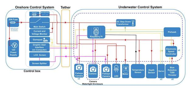
fig.6 Planned System Integration Diagram (SID)
