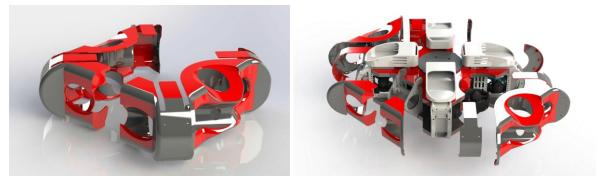
fig.12 The design of low drag streamlined body shell
