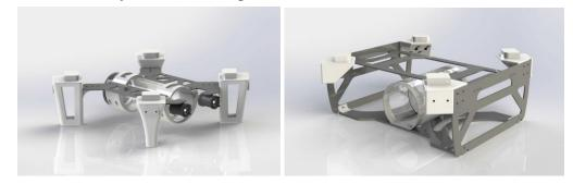
fig.8 Interchangeable tool plate CAD
