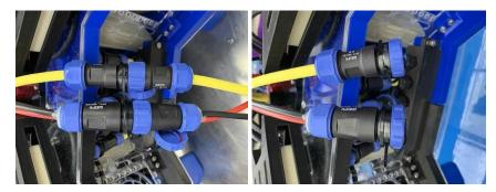
fig.7 Waterproofed quick-release plug
