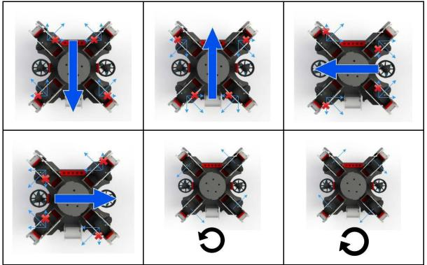
fig.13 The arrangement of thrusters leading to the multi-directional movement of the ROV
