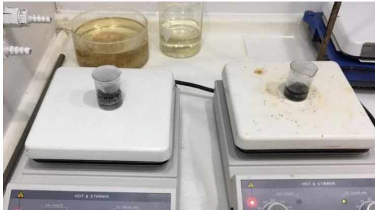
Figure 5. Impregnation process using ZnCl_2
