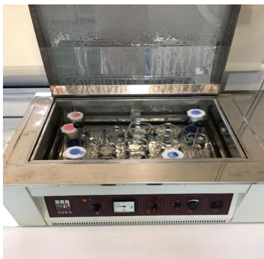
Figure 13. Water bath-thermostat shaker for adsorption trials.
