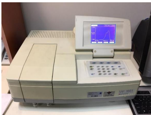
Figure 7. UV Visible Spectrophotometer (1601 Shimadzu) device.
