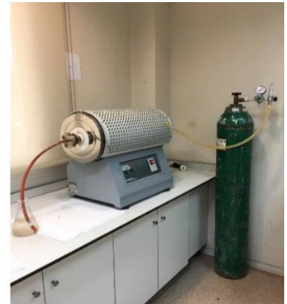
Figure 3. After pre-carbonization process (700°C, 30 minutes, N 2 ).
