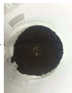
Figure 8: Magnetic particles after using a mortar to mash them.
