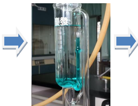
Figure 10: Soxhlet extractor was used to extract heavy metals from the polymers to form holes having the specificity toward copper ions.
