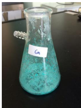
Figure 9: Copper polymers before the extraction of copper ions to form the molecular template.
