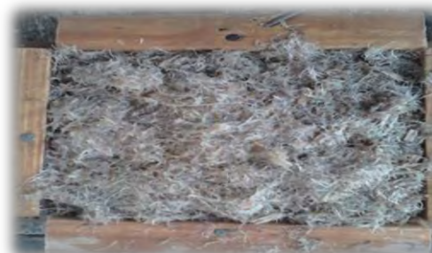
Figure 8. The fibers are subjected to a drying process
