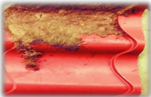
Figure 9 Molding step of the fibers to obtain biodegradable films
