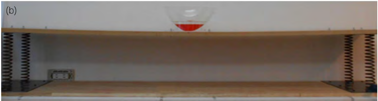
Fig. 2-1 (a) The shape of paraboloidal tank (b) The structure with a paraboloidal tank TLD
