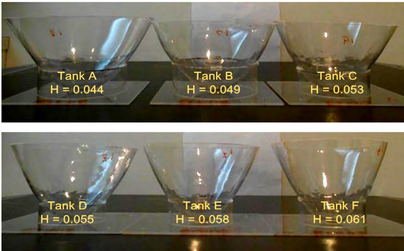
Fig. 4-2 Six different curvatures ( H = 0.044 \sim 0.061 ) of paraboloidal tanks (Tank A to F)
