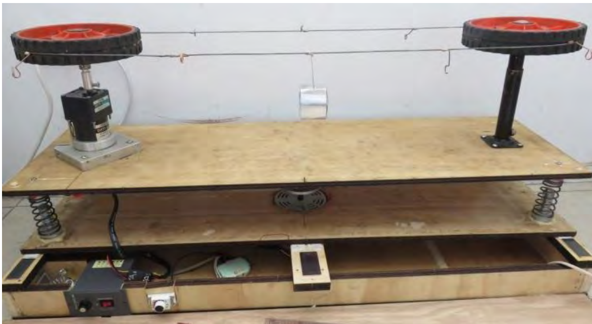
Fig. 22 The cable car system and earthquake simulator
