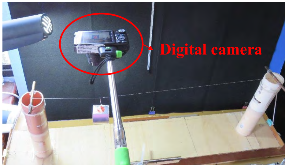
Fig. 7 Camera on the top of cable car system
