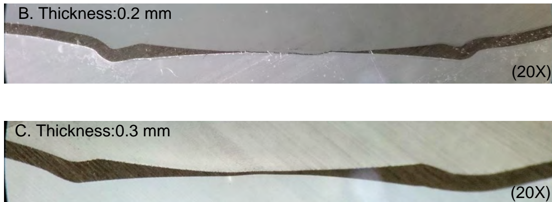
Fig. 34 Lateral views of collision patterns of single layer of aluminum foil
