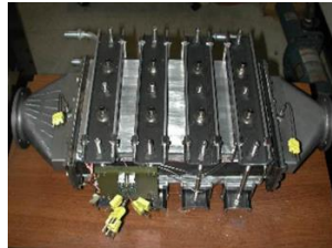
Figure 1-18: TEG used in automotive exhaust pipe actual situation [25]
