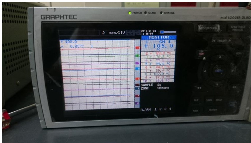
Figure 3-78: the 10 points of T_c and T_h in the measurement of 2 nd FTEM at current = 2A
