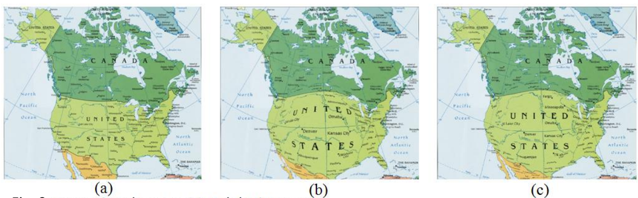
Fig. 9 Exemplary images (a) Original Image. (b) Fish-eye lens like magnification. (c) Fish-eye lens like magnification without distortion in central region.
