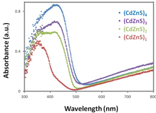
(B) Type 2:  $(\text{CdZnS})_{1\sim 4}/(\text{CdZnSe})_2$
