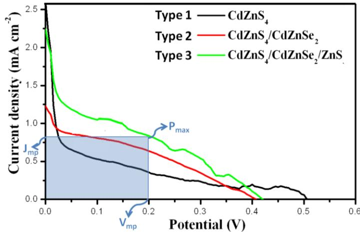
**Fig. 6 J-V curves of different sets of solar cells**
