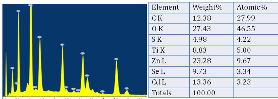
圖6  $\text{TiO}_2/(\text{CdZnS})_4/(\text{CdZnSe})_2/\text{ZnS}$  EDS分析
