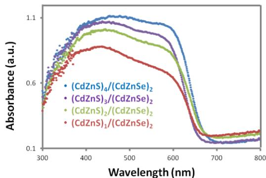
**Fig. 4 Absorption spectra of three types of QDs**
