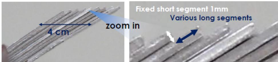
Fig. 3 Side views of the bound aluminum chips
