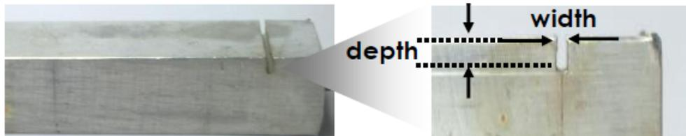
Fig. 5 Side views of an aluminum bar which has a notch with arrows to define the width and the depth of the notch
