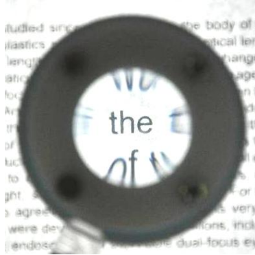
Fig. 11 The lens image with spherical aberration
