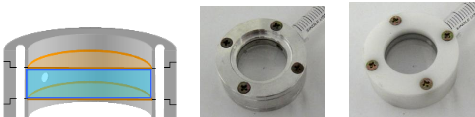
Fig. 7 Designed liquid lens of Generation 4 (left) and 4.5 (right)
