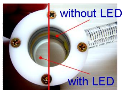
Fig. 29 The micro LED light can provide clear object image
