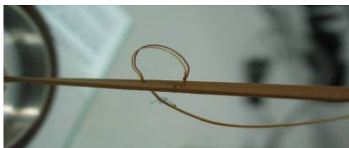
Fig. 2 A pair of thermocouple inserted into the rubber (left); the differential method for temperature measurement \Delta T with precision \sim 0.001^\circ\text{C} .
