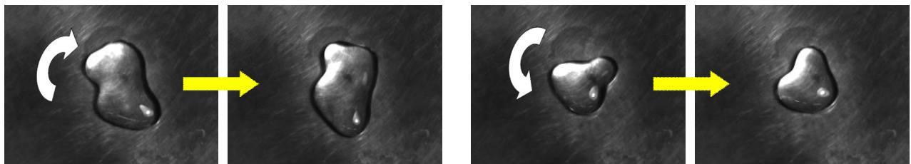
Figure 20. The observation of rotation of droplets on the hotplate. Both clockwise and anti-clockwise rotations can be observed as shown.
