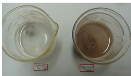
Fig. 5 The reaction of \text{H}_2\text{O}_2 with \text{Fe}_2\text{O}_3 -argil and argillaceous catalyst (Fe-A1-SiO 2 )
