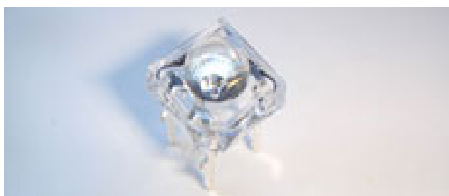
圖 5. 5mm Super Flux LED V_F(V)I_f=20mA (2.9V—3.5V) I_V(mcd)I_f=20mA (3300—4000)
