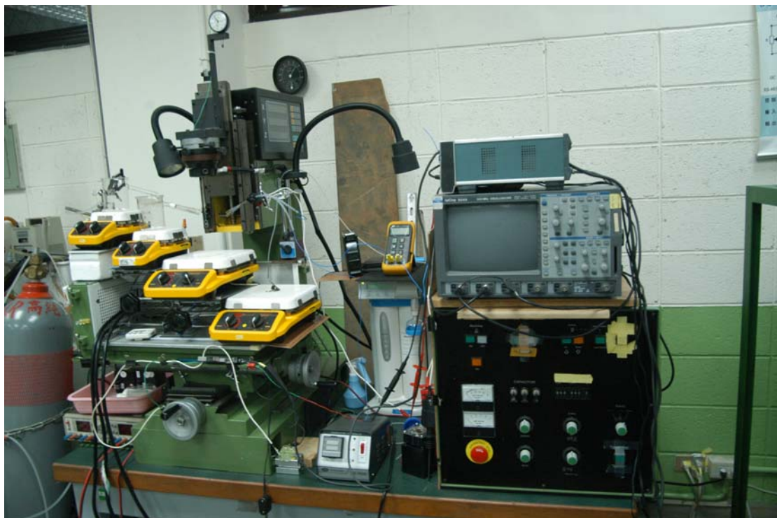
照片 6 膠體金粒子潛弧合成系統 (Picture 6 Au-NPs is produced by SANSS)
