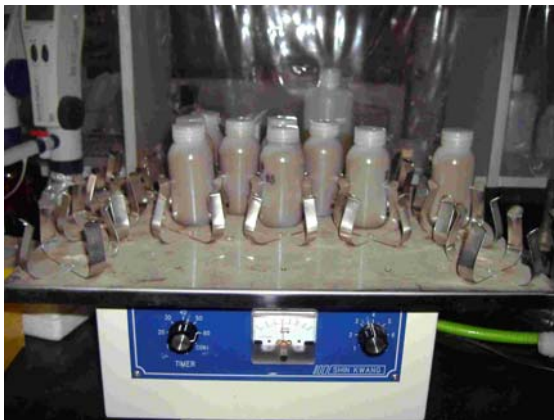
圖九 泥岩樣本於震盪器上震盪
