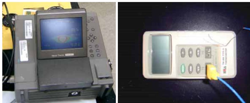
Picture 7 Left: Avio Handy Thermo TVS-100 Infrared Thermography. Right: Hola TM-906 K-type thermocouple.
