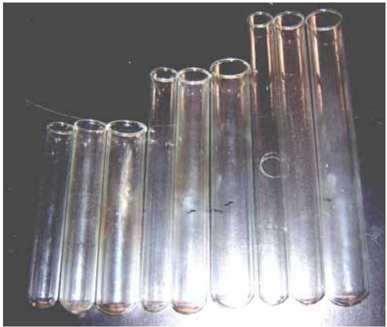
Picture 5 Nine Pyrex test tubes with lengths of 15, 20, 25cm, and diameters of 1.5, 2, 2.5cm.
