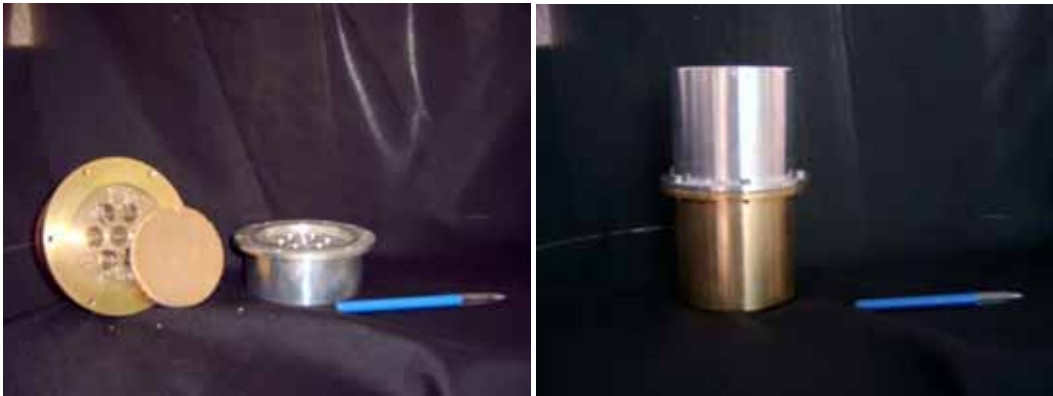
Picture 9 Passive TA cooler prototype (Mark I). Left: Components of prototype, copper and aluminum caps and ceramic stack. Right: Assembled device.
