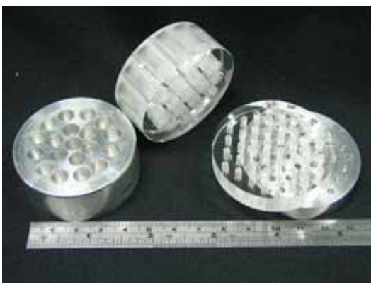
Picture 10 Passive TA cooler prototype (Mark II). The stack is integrated in the acrylic cap bringing the total components down to two, further simplifying fabrication.
