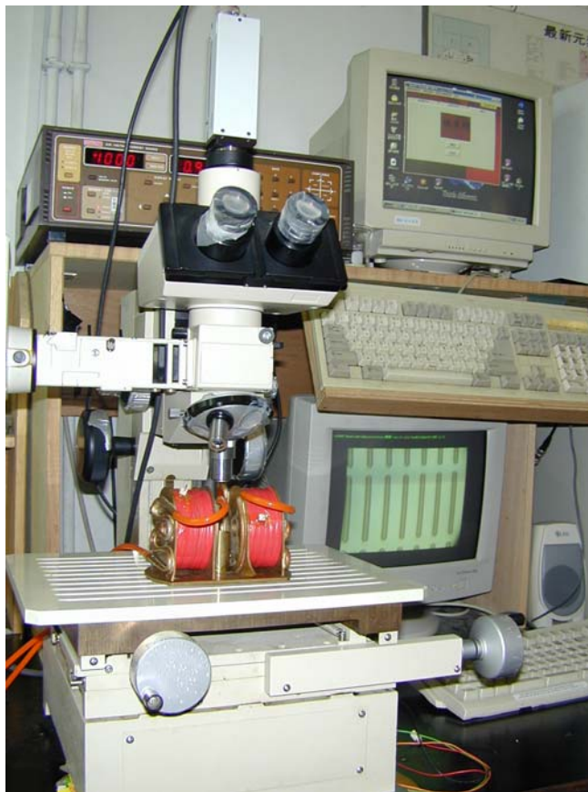
Fig.3. The device arrangement in the experiment for the ordered structure of the magnetic fluid film
