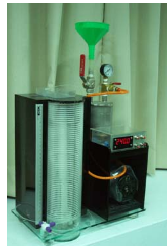
Photo. 1. Gravity sloping helical capillary viscometer
